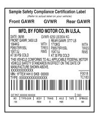
Exceeding the Safety Compliance Certification Label vehicle weight rating limits could result in substandard vehicle handling or performance, engine, transmission and/or structural damage, serious damage to the vehicle, loss of control and personal injury.
